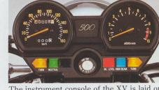
The instrument console of the XV is laid out in simple, easy-to-read fashion. It includes speedometer, electric tachometer, odometer with re-settable trip meter and indicator lights for major machine functions. The main ignition switch also incorporates a steering lock as an additional theft deterrent.
