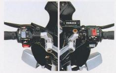
The beautifully finished, forged aluminium handlebars are lighter and more rigid than normal tubular components. Even more important, they allow complete adjustability for arm reach and handlebar grip angles to suit the individual rider.
