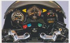
The centrally-mounted tachometer is the focal point of the aircraft-style, triple meter instrument console. Also incorporated in this unit are speedometer, odometer, fuel gauge, digital clock and machine function warning lights.
