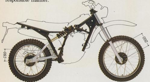
The Monocross suspension is derived directly from Yamaha's World Championship-winning motocrossers. It provides impeccable handling on or off the road, thanks to the 180-mm wheel travel by the single De Carbon type damper. The triangulated swing arm using box-section tubing is built strong, eliminating rear wheel flex.
