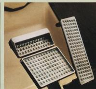
Extra large spike proof pedals. Stopping and parking brake combined on one pedal for simplest operation.
