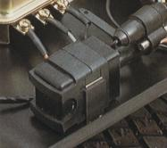
CDI Solid State Ignition never needs a tune-up. No points to burn out. No condenser to replace. Timing never goes out. Another Yamaha first.
