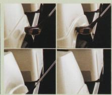
Tough, resilient front cowl will not chip or crack. Resininjected high-impact urethane springs back to its original shape again and again in gruelling crash test trials.
