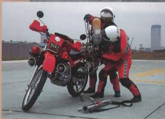
(Above) The Serow 225s serve as "Quick Attacker" units at five local fire departments around Tokyo. (Left) The "Quick Attacker" mounts a portable fire extinguisher known as an "impulse spray gun" on its special carrier. — From Tokyo Fire Department's "Catastrophe Response Training."
