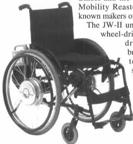
The JW-II units to be supplied consist of two wheel-drive assemblies containing all the drive mechanisms, attachment brackets, a battery and a special battery charger and include some specification modifications to fit European safety regulations and conditions of use. The battery provided is a newly developed Nickel-hydrogen type.
