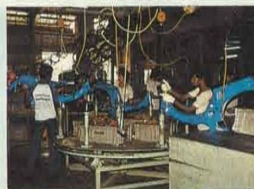
Taillamps being attached to the frame
