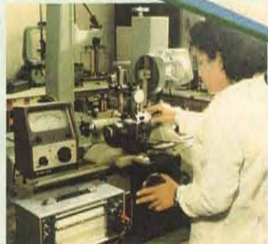
Each piston is precisely inspected for its shape.
