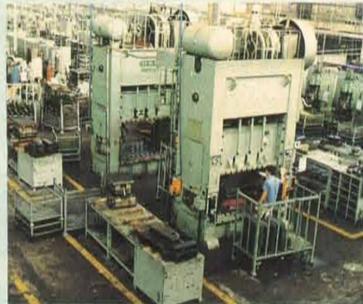
Press work for fuel tanks and mufflers etc.
