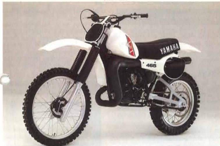
• Engine: 2-stroke single • Displacement: 465cc • Bore x stroke: 85 x 82mm • Compression ratio: 7.0 : 1 • Max. power output: 52hp (7,000rpm) • Max. torque: 5.75kg-m (6,000rpm) • Carburetor: 1-Mikuni VM38 • Ignition: C.D.I. • Starting: kick • Lubrication: pre-mix • Transmission: 5-speed gearbox • Seat height: 950mm • Wheelbase: 1,480mm • Dry weight: 104kg • Front tire: 3.00-21 • Rear tire: 5.10-18
