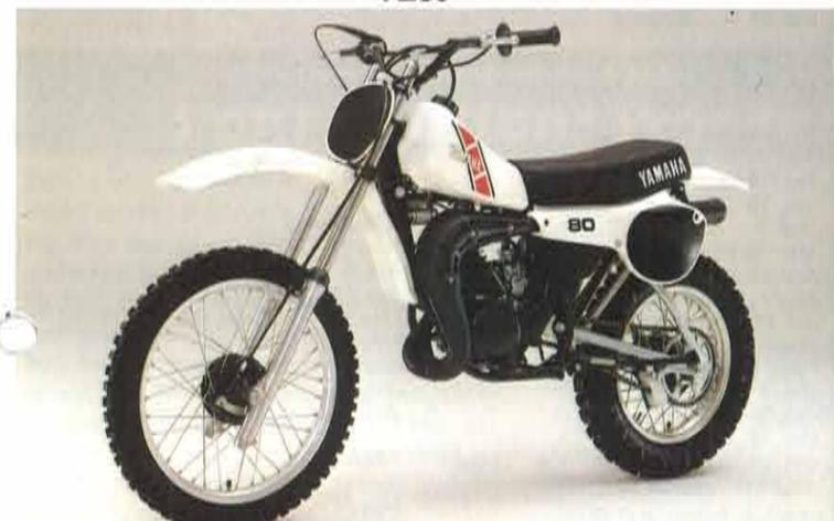
• Engine: 2-stroke single • Displacement: 79cc • Bore x stroke: 49 x 42mm • Compression ratio: 7.1 : 1 • Max. power output: 17hp (11,500rpm) • Max. torque: 1.06kg-m (11,000rpm) • Carburetor: 1-Mikuni VM26SS • Ignition: C.D.I. • Starting: kick • Lubrication: pre-mix • Transmission: 6-speed gearbox • Seat height: 760mm • Wheelbase: 1,205mm • Dry weight: 60kg • Front tire: 2.75-17 • Rear tire: 4.10-14
