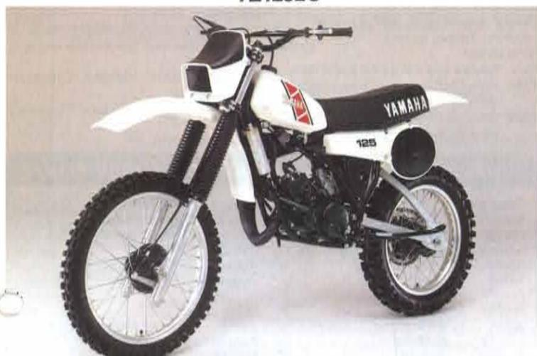
• Engine: 2-stroke single • Displacement: 123cc • Bore x stroke: 56 x 50mm • Compression ratio: 8.5 : 1 • Max. power output: 30.0hp (10,500rpm) • Max. torque: 2.04kg-m (10,000rpm) • Carburetor: 1-Mikuni VM32SS • Ignition: C.D.I. • Starting: kick • Lubrication: pre-mix • Transmission: 6-speed gearbox • Seat height: 945mm • Wheelbase: 1,450mm • Dry weight: 89kg • Front tire: 3.00-21 • Rear tire: 4.00-18
