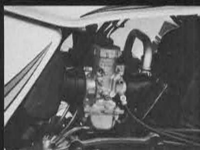
A balance pipe links both intake tubes to increase power output over the range of low-to-medium rpm's.
