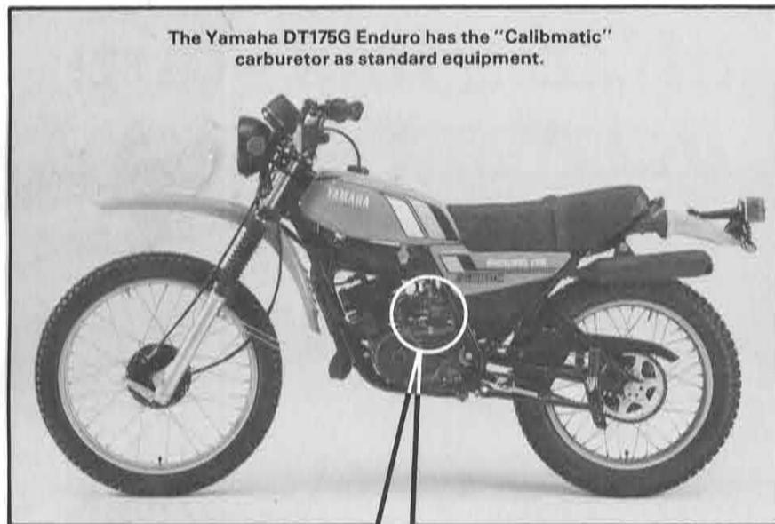
The Yamaha DT175G Enduro has the "Calibmatic" carburetor as standard equipment.
