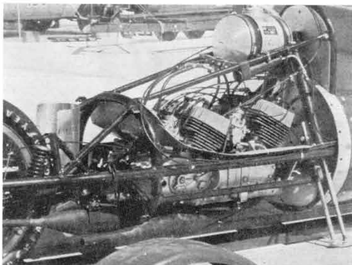
▲ The two 350cc TR-2 engines are coupled neatly into one unit. (Reproduced from Motor Cycle)
