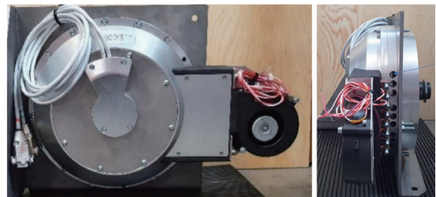
Fig. 11 EVT Machine (An angle sensor is visible in the center of the cylinder side, but this may be eliminated to achieve a sensorless design.)
