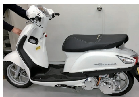
Fig. 26 Exterior View of Vehicle Fitted with Series Hybrid
