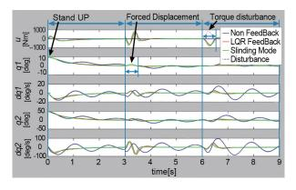
Fig.15 Feedback simulation
