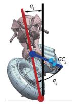
Fig.5 Center of gravity difference
