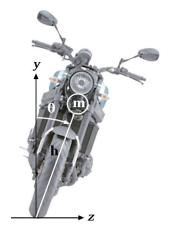
Fig.1 Inverted pendulum model
