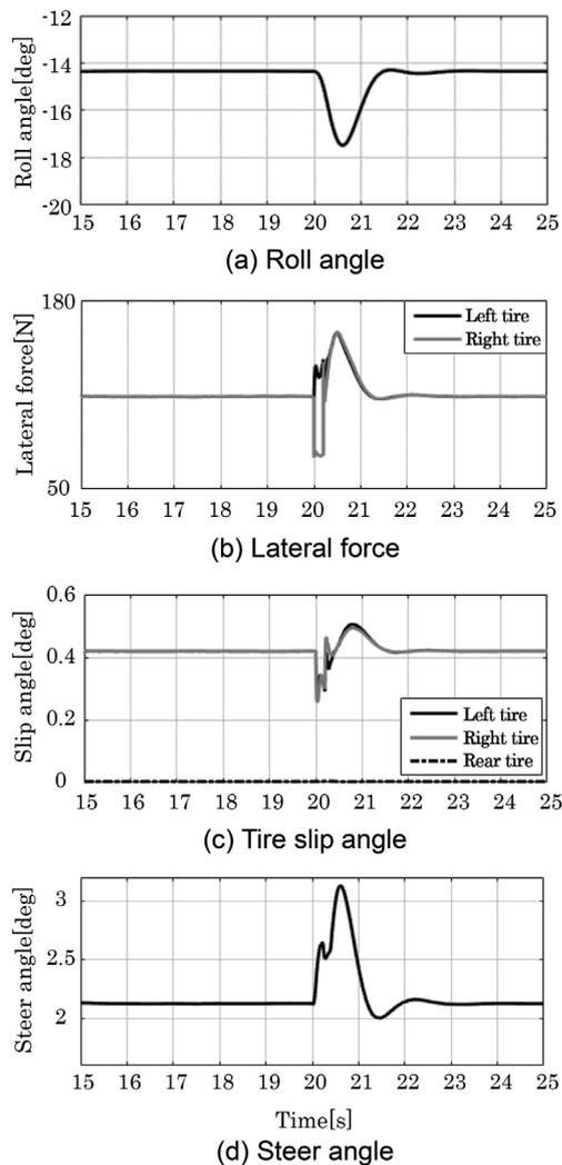
Fig.19 Analysis Results with No Steering Torque Control
