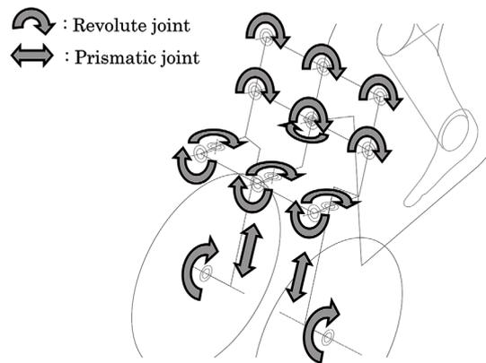
Fig.9 Lean Mechanism of the Simulation Model
