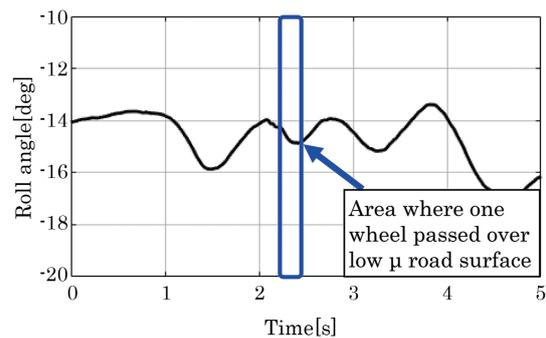
Fig.5 Roll Angle Measurement Data at Left Turn
