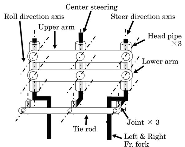
Fig.10 Detailed Drawing of the Lean Mechanism
