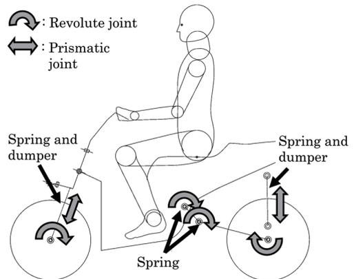
Fig.8 LMVW Simulation Model
