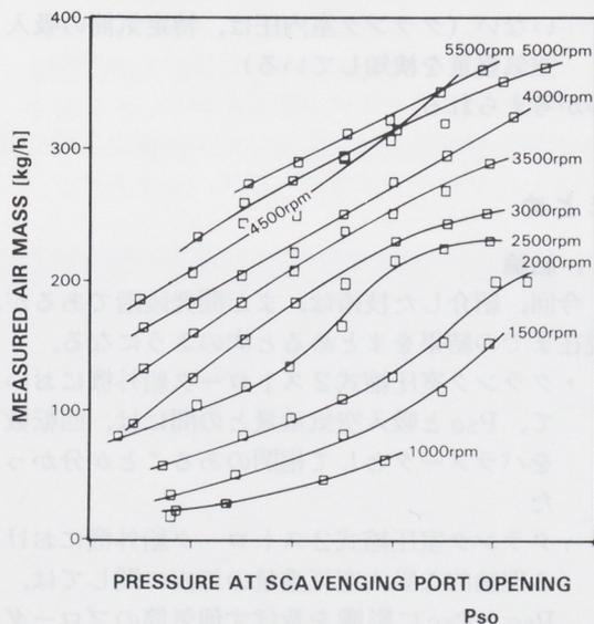
Fig 7 Correlation between corrected theory and Measured Data.
