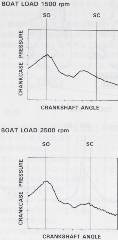
Fig 6 Crankcase Pressure Waveform.
