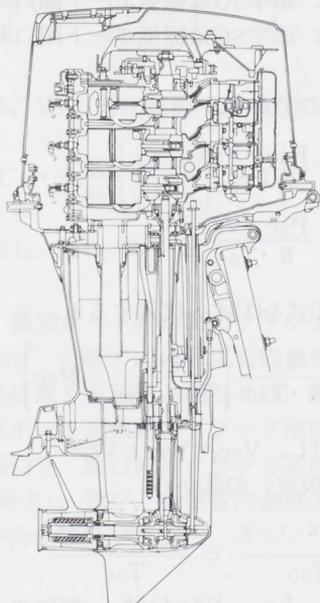
Fig 2 Vertical Section of the model YAMAHA 90ATE.
