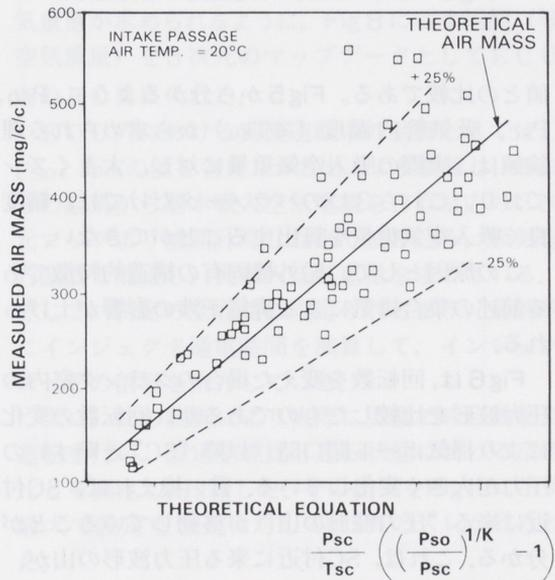
Fig 5 Correlation between theory and Measured Data.
