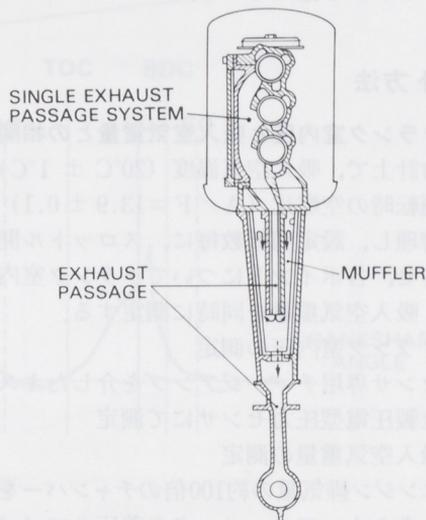
Fig 3 Sectional view of exhaust.
