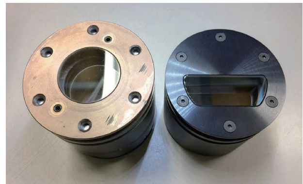
Fig. 2 Visualization piston; Right is used in this study and left is used in previous study.
