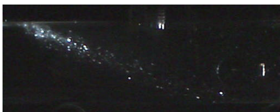
Fig.25 Spray picture (n-heptane, 40 m/s, 90 C, 7.5 ms)
