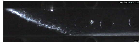
Fig.16 Spray picture (n-heptane, 40 m/s, 60 C, 7.5 ms)
