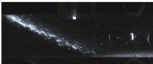
Fig.22 Spray picture (n-heptane, 40 m/s, 25 C, 7.5 ms)
