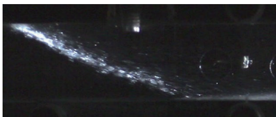
Fig.23 Spray picture (n-heptane, 40 m/s, 60 C, 7.5 ms)
