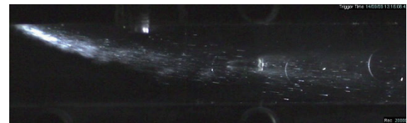
Fig.17 Spray picture (n-heptane, 60 m/s, 60 C, 7.5 ms)
