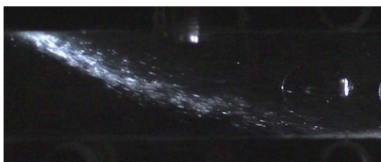
Fig.24 Spray picture (n-heptane, 40 m/s, 90 C, 7.5 ms)
