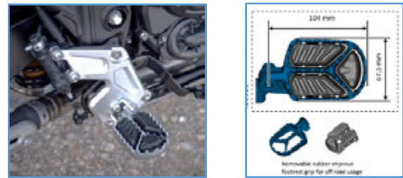
Fig. 10 Wide Foldable Foot Pegs with Removable Rubber
