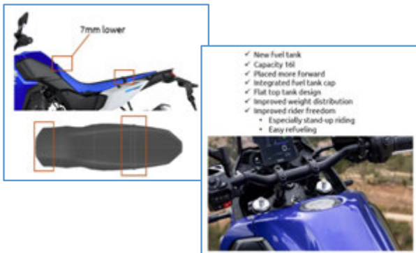
Fig. 6 Seat: One Piece Rally Seat and New Fuel Tank Design
