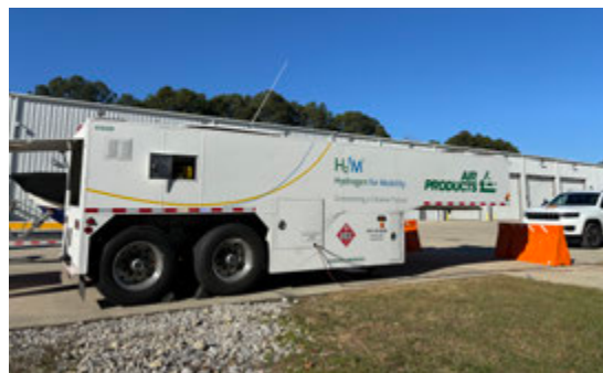
図26 移動式水素供給装置 (Air Products HF-150)
