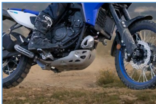
Fig. 8 Aluminium Skid Plate and Ground Clearance
