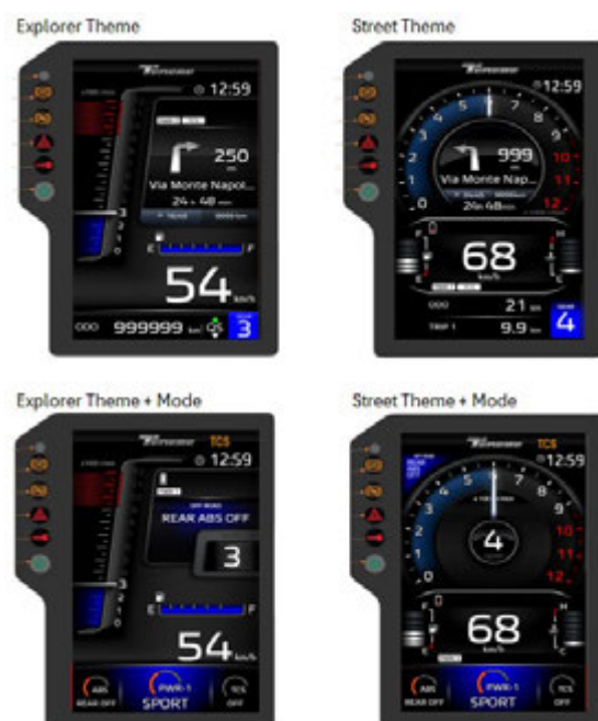
Fig. 19 Meter, 6.3-Inch Vertical Meter and Connectivity Features
