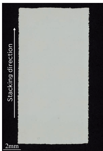
Fig. 5 Cross-sectional view of specimen fabricated with optimal parameters
