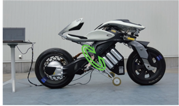
Fig. 6 Experiment applying a disturbance to the AMCES shaft
