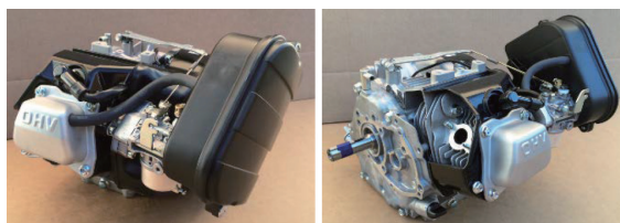
Fig.2 MZ200SMB improved for fitting to the Snoscoot
