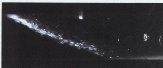
Fig.23 Spray picture (n-heptane, 40 m/s, 60 C, 7.5 ms)
