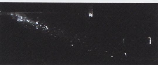
Fig.25 Spray picture (n-heptane, 40 m/s, 90 C, 7.5 ms)
