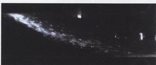
Fig.24 Spray picture (n-heptane, 40 m/s, 90 C, 7.5 ms)
