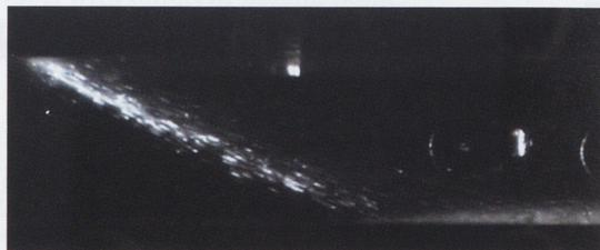
Fig.22 Spray picture (n-heptane, 40 m/s, 25 C, 7.5 ms)
