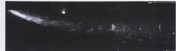
Fig.17 Spray picture (n-heptane, 60 m/s, 60 C, 7.5 ms)
