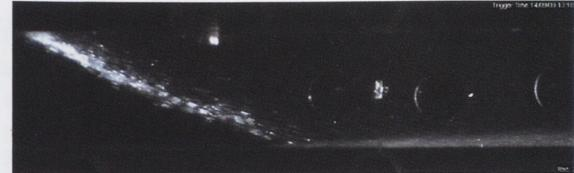
Fig.16 Spray picture (n-heptane, 40 m/s, 60 C, 7.5 ms)
