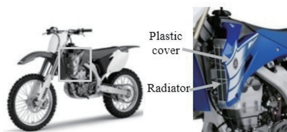
Figure 1: Appearance of radiator and plastic cover
