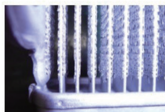
Figure 11: Radiator without fins
