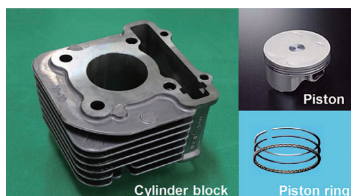
Figure 6: Appearance of tested components, cylinder block, piston and piston rings.
