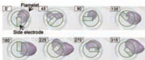
Figure 5: Simulated flame expansion (effect of plug direction)
