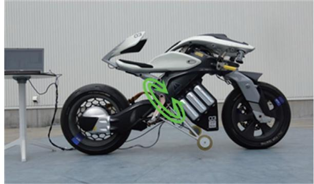
Fig. 6 Experiment applying a disturbance to the AMCES shaft
