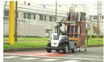
*eve auto* being used outdoors for automated transport of parts between factory buildings
