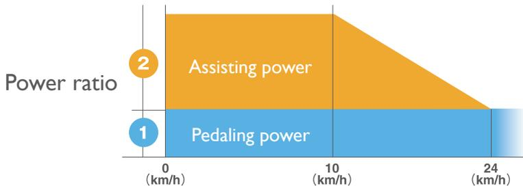
Up to 10 km/h, electric power assists pedaling at a maximum ratio of 1:2\*
