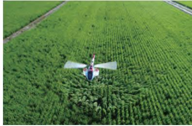
Aerial agrichemical spraying using unmanned helicopter
