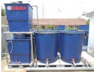
With the help and coordination of public and international bodies and institutions, Yamaha Motor is building and installing water purification systems in areas with limited or no access to potable water—primarily in small villages in Africa and Southeast Asia—in order to improve the quality of life.
