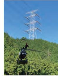
Logistics transportation using GPS-based automatic navigation
