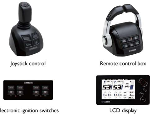
The Helm Master digitally controls all the steering, gear shifting and throttle work of twin or triple mount large-class Yamaha outboards. Complementing the standard steering and remote control unit, the single joystick control enables fore-aft, port-starboard and diagonal motion as well as in-place rotation of the bow.
