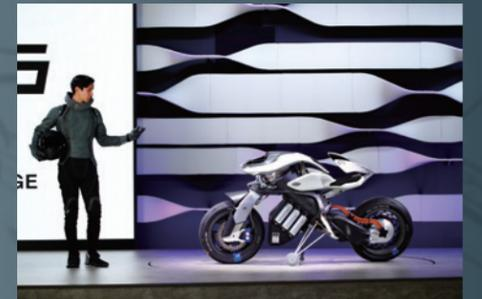
Image Recognition AI: A facial recognition system gives MOTOROiD the ability to respond only to its owner. It is also able to recognize gestures, making it possible for MOTOROiD to respond to hand movements as well, like using a beckoning wave or a raised palm to instruct it to start or stop moving.
