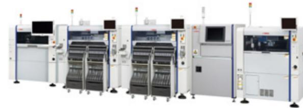
Mounter line centered on high-end, highly efficient modular Z-LEX YSM20R
