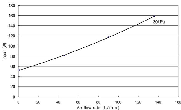
Fig. 2 Air pump electricity consumption
