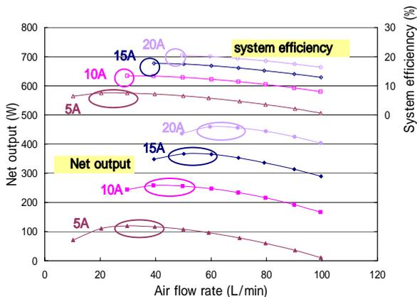
Fig. 8 Air flow in relation to net output and system efficiency
