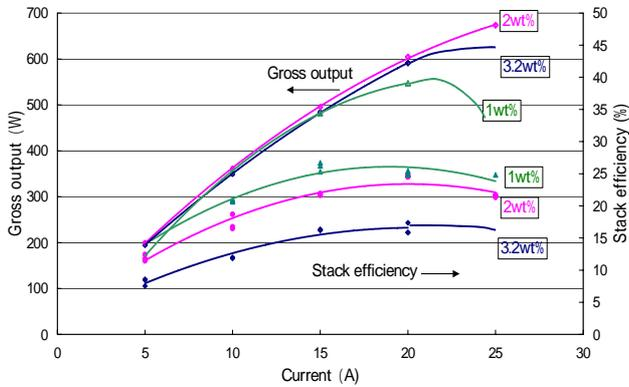
Fig. 4 The relationship between cell stack gross output and efficiency and amperage at the different fuel-water solution concentration levels.
