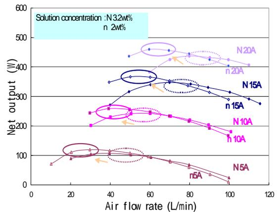
Fig. 6 The relationship between air flow rate and net output
