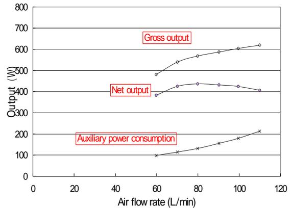
Fig. 5 The dependency on air flow for DMFC output @ 20ACC operation
