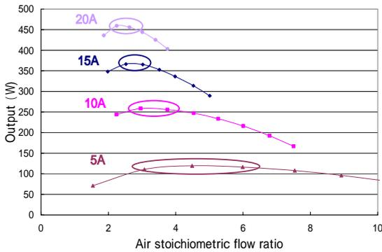
Fig. 7 The relationship between air stoichiometric rate and net output
