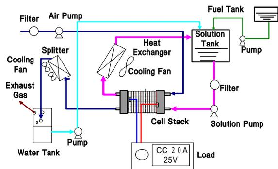
Fig.1 Configuration of the test set-up
