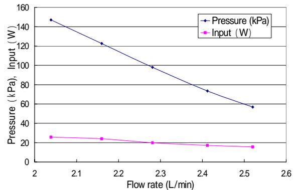
Fig. 3 Characteristics of the solution pump
