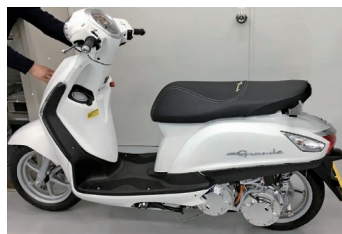
Fig. 26 Exterior View of Vehicle Fitted with Series Hybrid
