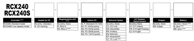
Note 1. The RCX240S controller is limited to use with robots that handles 200W or lower on each axis. Check the following controller selection table to find the matching model.
