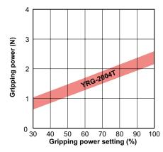
Graph shows a general guide to gripping power versus gripping power setting (%). Variations will appear in the actual gripping power
