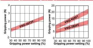
• Graph shows a general guide to gripping power versus gripping power setting (%). Variations will appear in the actual gripping power.
