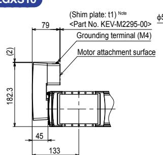
Note. For the availability of shim plate, see the adaptable servo motor table (P.38).
