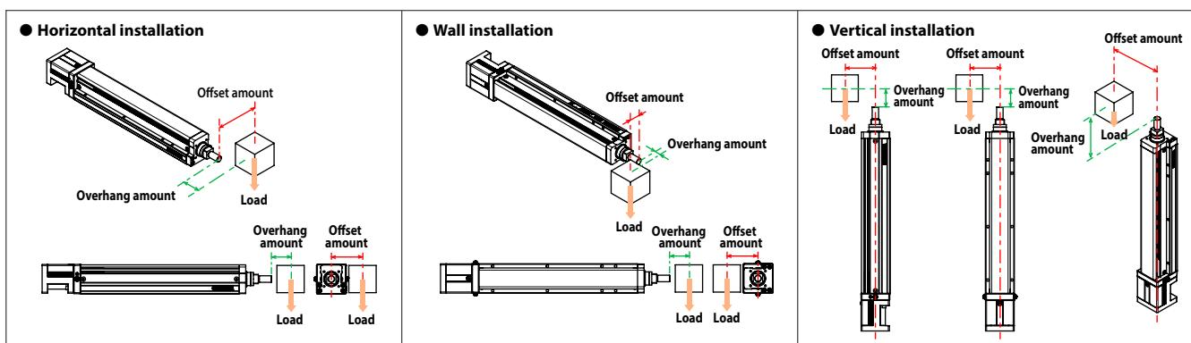
Note 1. When transferring an object with a weight exceeding the following, use an external support guide.
