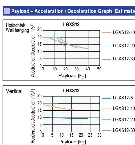
**Effective stroke and maximum speed during high acceleration or deceleration**
