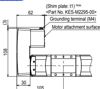
Note. For the availability of shim plate, see the adaptable servo motor table (P.32).
