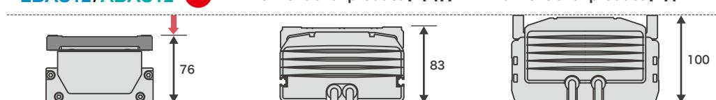
With the same frame width, the product can be used for both 200W and 400W motors, making it suitable for a wide range of situations.
