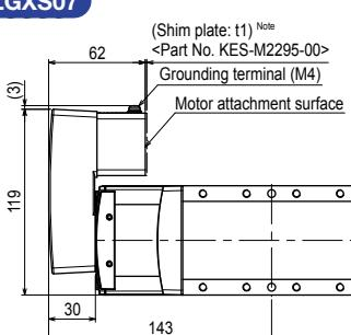
Note. For the availability of shim plate, see the adaptable servo motor table (P.36).
