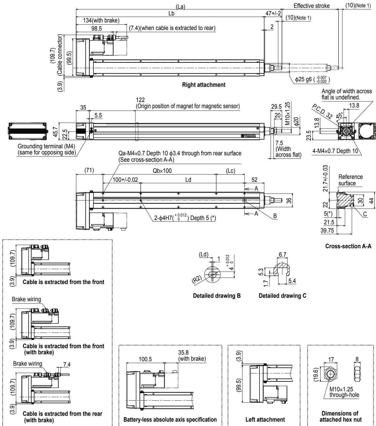
Note 1. Stop positions are determined by the mechanical stoppers at both ends.
