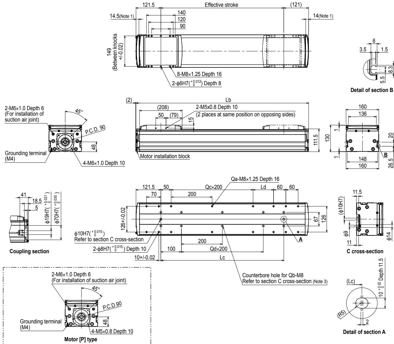
Note 1. Stop positions are determined by the mechanical stoppers at both ends.
