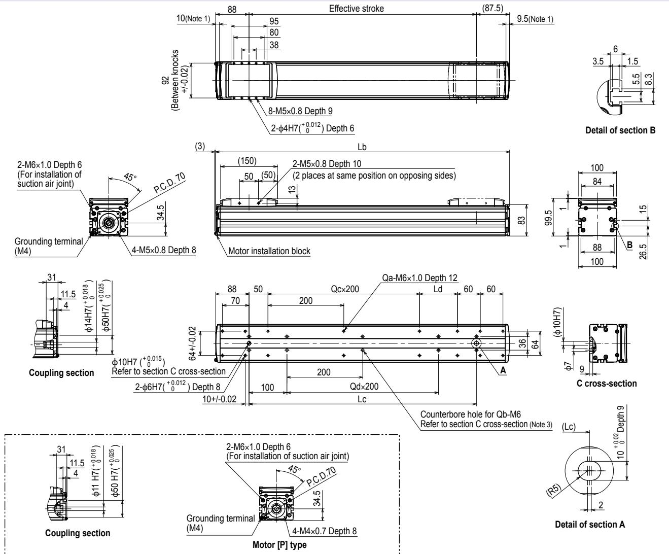
Note 1. Stop positions are determined by the mechanical stoppers at both ends.
