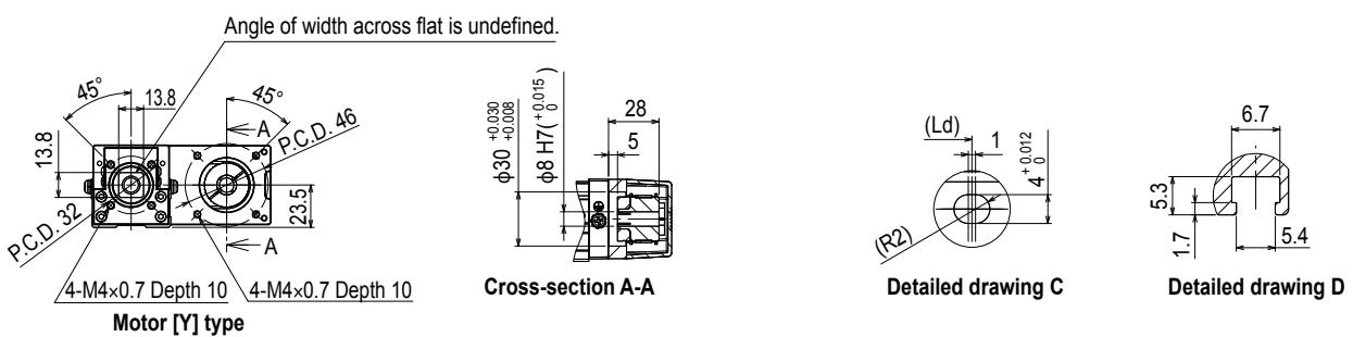
Note 1. Stop positions are determined by the mechanical stoppers at both ends.
