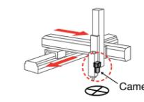
If camera is fixed, attach fiducial mark to robot, and move it
