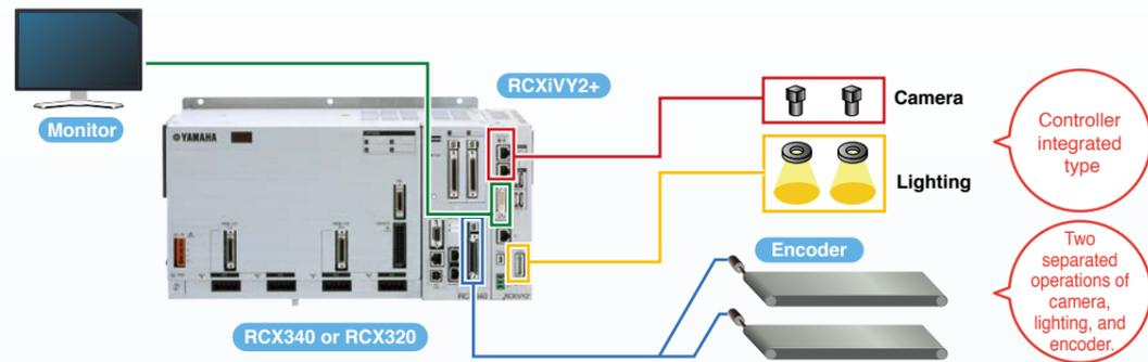
Typical Robot Vision setup
