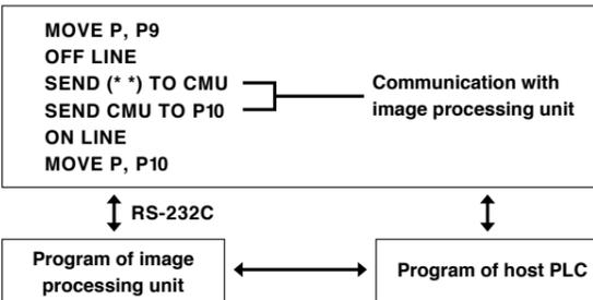
Camera and robot have separate programs
