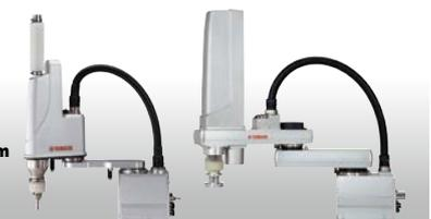
This model is designed for work environments involving frequent water splashing and dust (with the protection class being equivalent to IP65).
