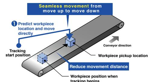
Operating conditions: YK500XG / payload 1 kg (total of workpiece and tool) / horizontal movement 250 mm / vertical movement 1 mm / conveyor speed 100 mm/sec
