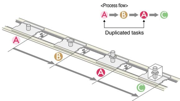
**LCMR200 / LCM100** Eliminating duplicated work station
