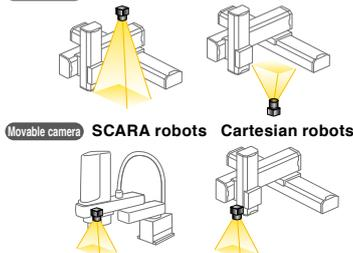
Even when the camera is moved, the coordinates are corrected automatically.
