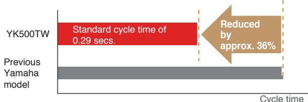
The standard cycle time for moving a 1-kg load 300 mm horizontally and 25 mm vertically has been reduced by approximately 36% compared to older Yamaha models.
