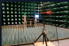
\* Our anechoic chambers have been set up to help us in the overall development of EMC (Electro-Magnetic Compatibility) technologies deployed in products produced by Yamaha Group companies. This allows us to ensure compliance with international regulations and conformity with international standards.
