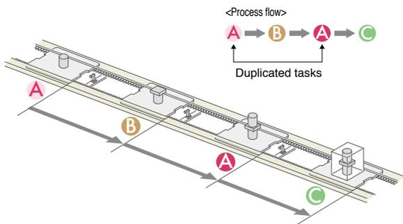
**LCMR200 / LCM100** Eliminating duplicated work station
