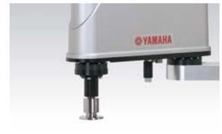
Tool flange option for easy mounting of a tool to the tip
