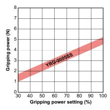
Graph shows a general guide to gripping power versus gripping power setting (%). Variations will appear in the actual gripping power.
