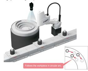
· Vision tracking and sensor tracking are supported.
