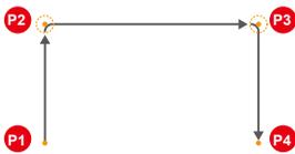
Normally, P1 to P4 are specified. Each operation starts the next operation when it enters the out enable position range.
