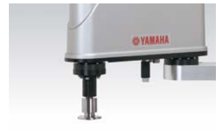
Tool flange option for easy mounting of a tool to the tip Note: YK250XG to YK1000XG
