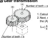
1. Calculate the moment of inertia  $I_B$  around the (B) axis. 2. Next, substitute  $I_{\mbox{\scriptsize B}}$  for the moment of inertia around
