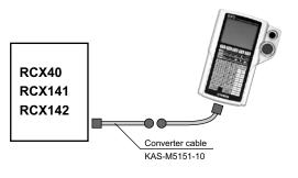
Converter cable for operating the RCX40, RCX141, RCX142 by RPB.
