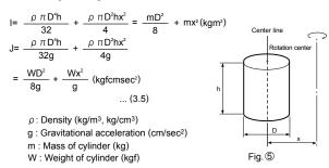
In the same manner, the moment of inertia of a cylinder as shown in Fig. 6 is given by
