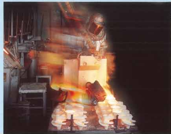
The lost-wax method allows propellers to be cast as single units. El método de cera perdida permite fundir las hélices una a una.
