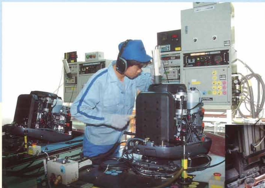
In the final inspection, each completed motor is actually started up to check all aspects of it. En la inspección final se hace arrancar cada motor terminado para comprobarlo por completo.
