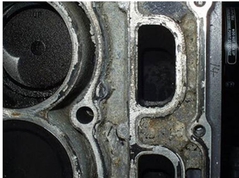
Flushing not performed (approximately 500 hours of usage)
