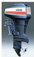
The 55A became the foundation for Yamaha's move into the large-horsepower category. Its liquid-cooled 2-cylinder 760cc engine had several unique technologies like a fully carburized one-piece crankcase, 2-piece connecting rods and more.
