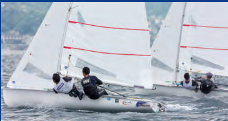
During testing, two boats are sailed together while gathering a variety of data for hull development.
