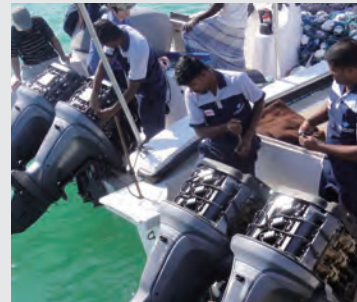
Performing service inspections on large-horsepower outboards (UAE)
