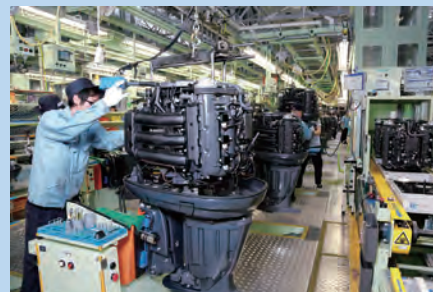
The final assembly process. Here components put together in the sub-assembly stages are assembled together precisely into the numerous model specifications
