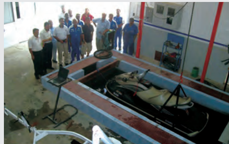
The new PWC test tank is equipped for simultaneous computer diagnostics
