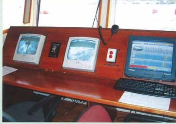
*With the modernization of the fish farming facilities, the timing and volume of feed distribution is now computer controlled and can be monitored from the control shed*
