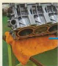
Example of protecting parts during work
