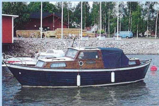
A traditional double-ender. Most are wooden boats with inboard motors.
