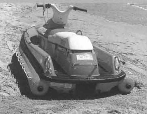
The WaveRunner 650 VXR is fitted with an inflatable hull and used as a surf rescue/patrol craft.
